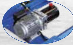
Powerful electric motor with hydraulic drive
