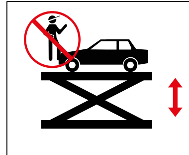
No objects or persons may be transported on the lifting platform, the support arms or on the vehicle to be lifted.
